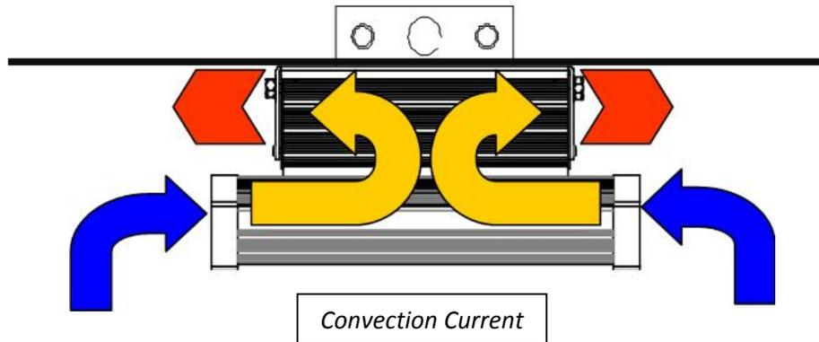
With passive cooling, plenum design relies on the basic principle that heat rises. Upward movement of heated air creates a low pressure that draws in fresh air to equalize the pressure. Robust plenum design provides an entry point for fresh air, a path through the convection surfaces, and an exit path for heated air to escape.
