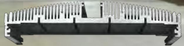
The housing design draws a plenum of fresh air from five sides. In addition to carrying heat from the LED array, the power supply sits on custom risers for six-sided convection. The result is the industry's lowest operating temperatures, a 67.1°C LED and 58.1°C power supply<sup>(1)</sup>. At the same time, the solid top covers against the effects of dust and birds.
